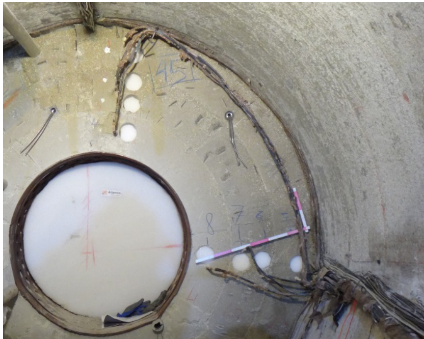
Fig. 64: Cores taken following the TDR sensors inside the bentonite buffer.
