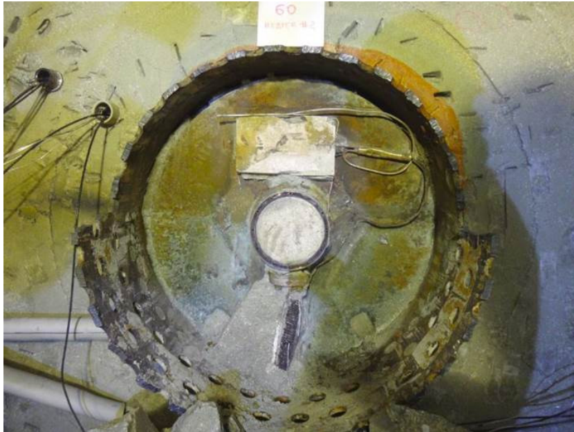
Fig. 46: View of the uncovered heater front.
