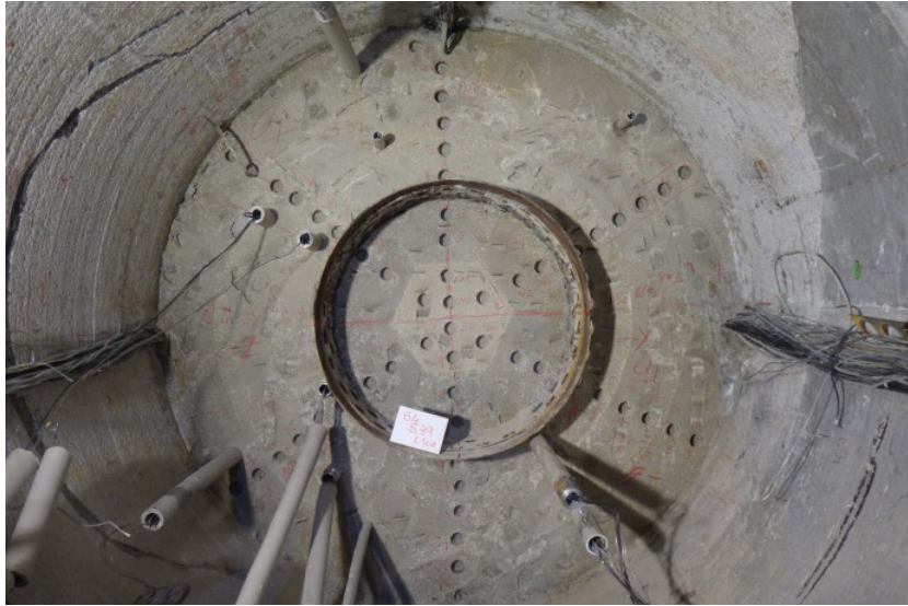
Fig. 42: View of bentonite layer 64 during dismantling.
