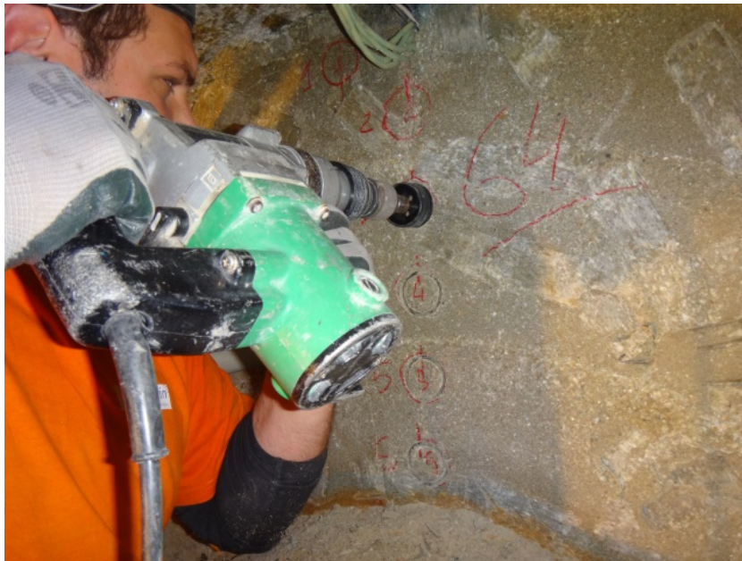
Fig. 74: Samples extraction with crown drill.
