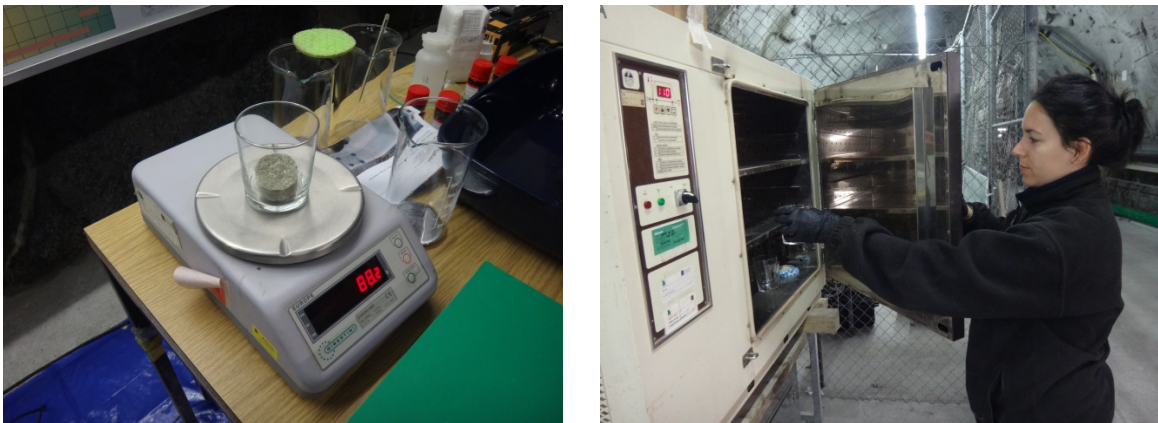
Fig. 77: Procedure for water content determination, weighting at the left hand side and introduction in the oven at the right.
