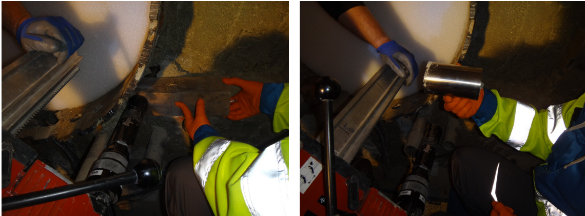
Fig. 62: Pushing of Shelby tubes while Sampling Section S42.
