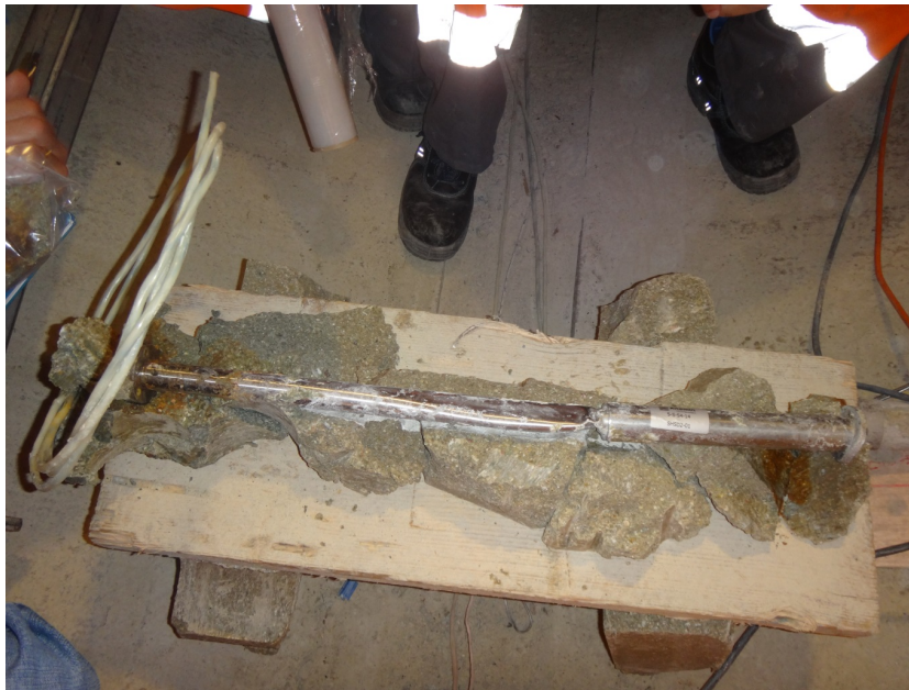
Fig. 67: Extensometer in S54 and reconstruction of samples behind it.
