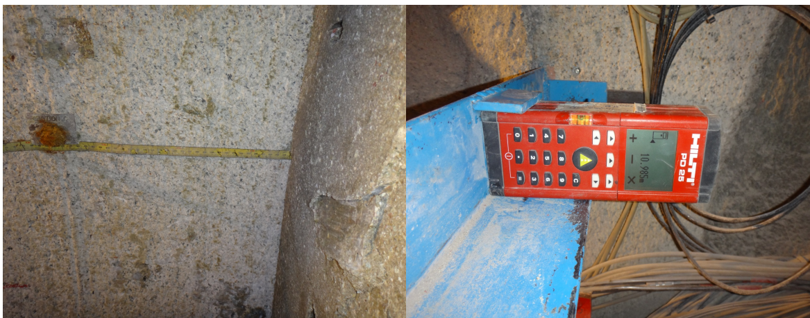
Fig. 39: View of the metric tape (left photo) and the laser device (right photo).
