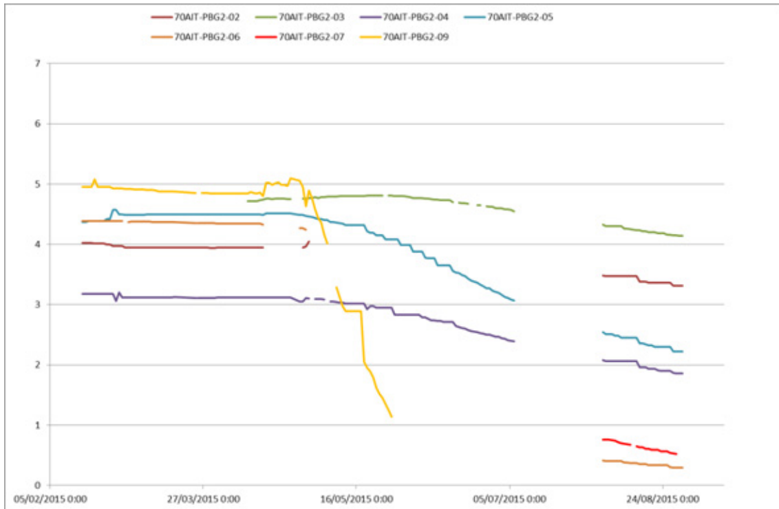
Fig. 8: Evolution of total pressures in borehole SG2 during the dismantling operation (MPa).
