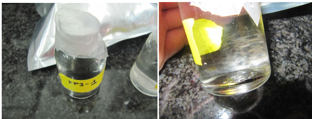
Fig. 65: Black particles observed at the bottom of the septum vial -1 from the FP3 pipe, which were analysed by scanning electron microscopy (SEM)
