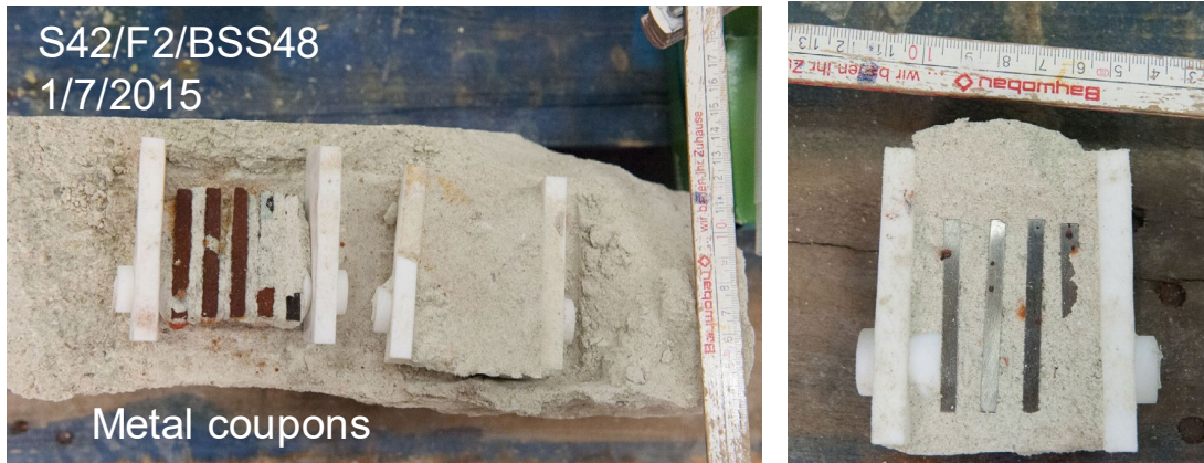
Fig. E-12: Metal coupons at Section 42 (Sampling Section BSS48/Instrumented Section F2)
