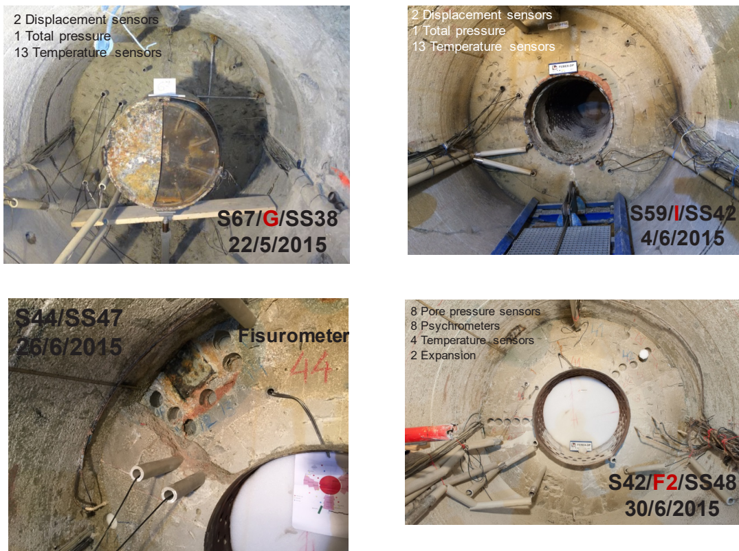
Fig. E-16: Visual aspect of the bentonite in the instrumented Sections G, I and F2 where the sintered filters for pore water sampling and RH measurements were located
