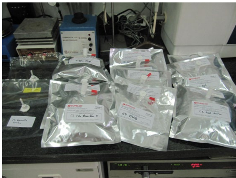
Fig. 104: Sampling bags with porewater collected from the CIEMAT pipes after their reception in the Pore Water Chemistry Laboratory at CIEMAT
