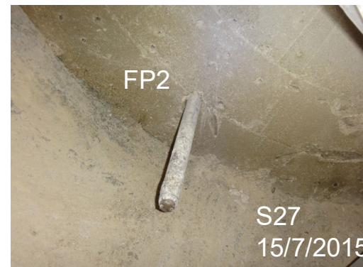
Fig. E-11: Visual aspect of the stainless steel pipes with no evidences of external corrosion
