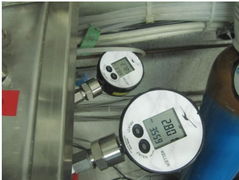
Fig. 60: LEX-1 type manometers: pressure measurements in the FPx-C/D lines while applying an overpressure in the sampling system for tightness checking of the sampling circuit.
