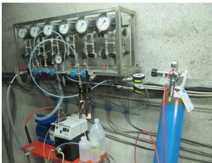
Fig. 37: Set-up of the system for collecting gas and water in the GRS pipes in 2014
