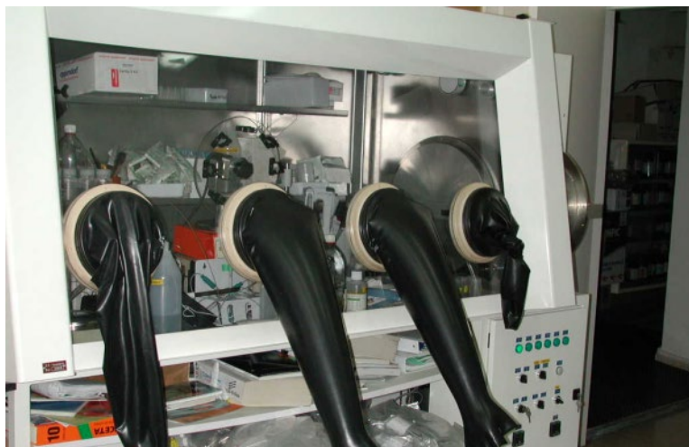
Fig. 46: Jacomex anoxic glove box ( < 1 ppm O_2 ) for pH and redox measurements in the porewaters from the FEBEX bentonite collected inside the sampling bags from the GRS and CIEMAT pipes
