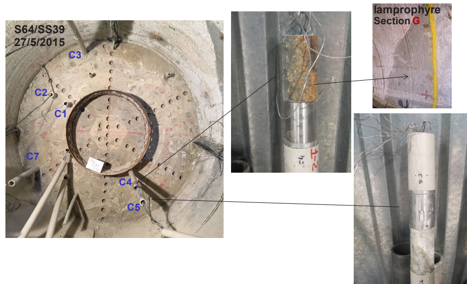
Fig. 54: Visual aspect of both the corroded sintered filter from pipe C4 and the non-corroded filter from the pipe C5 at Section G (close to a lamprophyre area)
