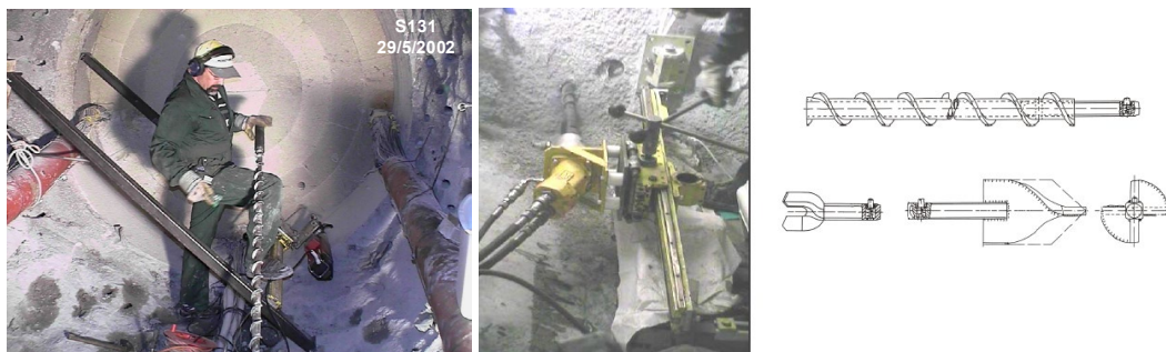
Fig. 28: Drilling machine, rod and bit used for drilling boreholes where the gas and water sampling pipes were inserted
