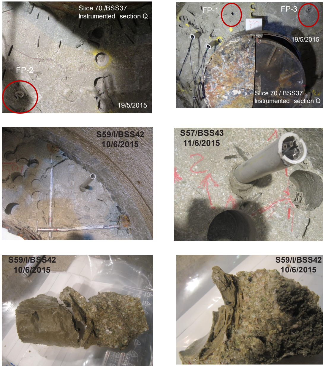
Fig. E-15: Gel of smectite generated around the pipe FP3, which was observed from the bentonite Slice 70 (BSS37, Instrumented Section Q) until the end of the tube (Section 52)
