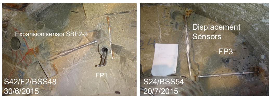
Fig. 51: Types of sensors potentially corroded and degraded in the bentonite barrier close to gas pipes FP-1, FP-2 and FP-3
