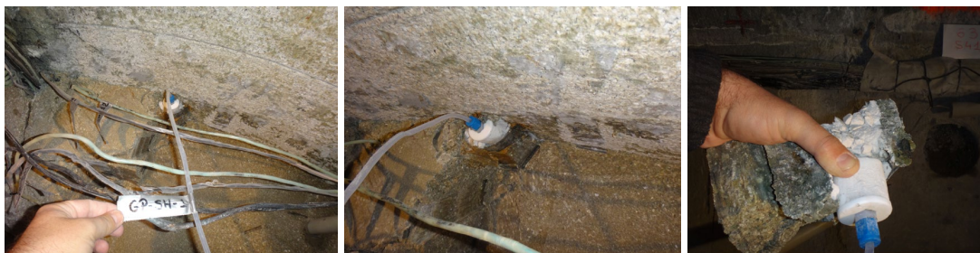
Fig. E-7: Visual aspect of the GRS pipe GP-S-H-3 for pore pressure measurements during the dismantling of the Heater #2 (29.05.2015) in the Slice 63 (BSS40, Instrumented Section H)
