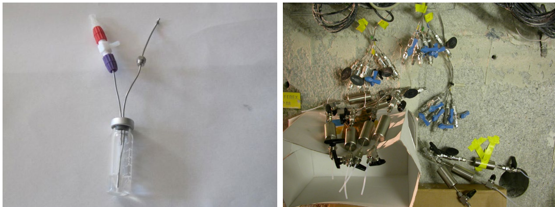
Fig. 45: Porewater sampling in CIEMAT pipes from 2006 to 2011: a) Septum vials. b) Stainless steel cylinders of 40 cm 3 with double end
