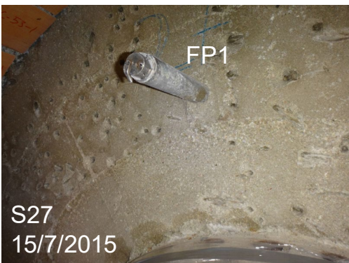
Fig. E-11: Visual aspect of the stainless steel pipes with no evidences of external corrosion
