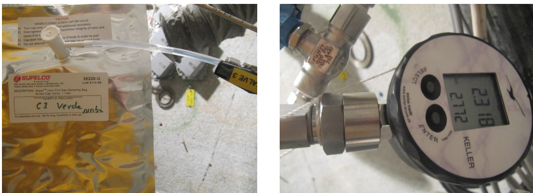
Fig. 107: Detail of the extraction of porewater from the pipe C3 at Section F2 (green colour) and detail of the corresponding interval pressure measurement
